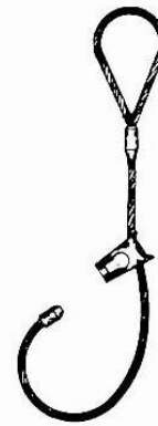
VLC1F/EOE 1 FERRULE/EYE ONE END
